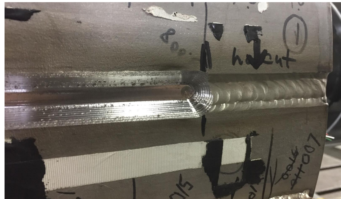
Iron lams test with magnetic powder
