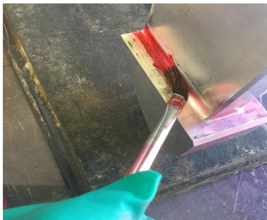
Al clamps test with die penetration technique
