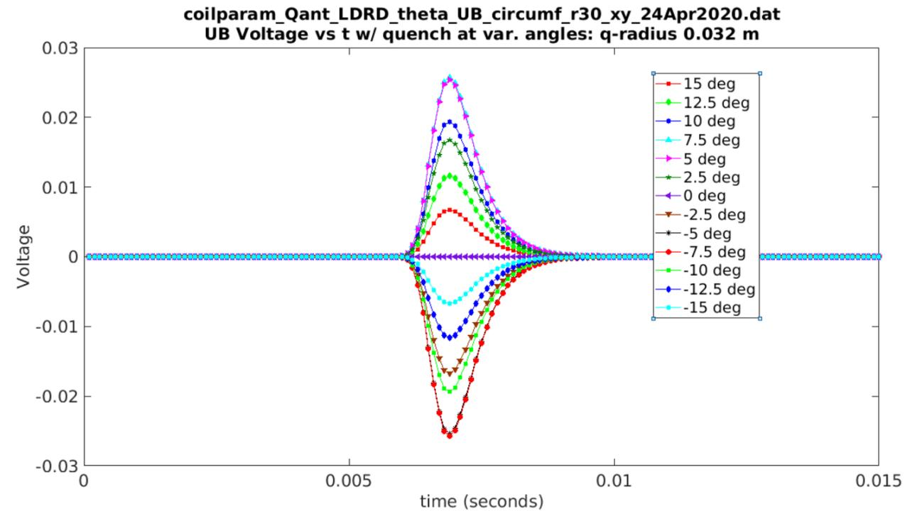
Large signal – quench is very close to antenna
