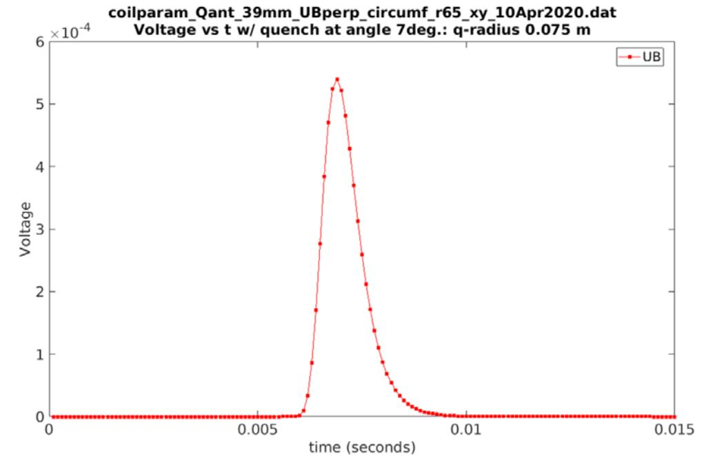
Simulation model recreates fairly well the response (including magnitude) of the experimental quench antenna voltage signal data (both parallel and perpendicular) taken at known quench location on MQXFS1.
