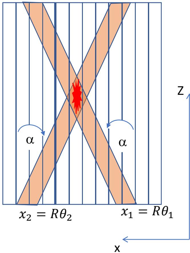
Use intersection of determined quench angle/x-position from each of the two panels to locate quench.
