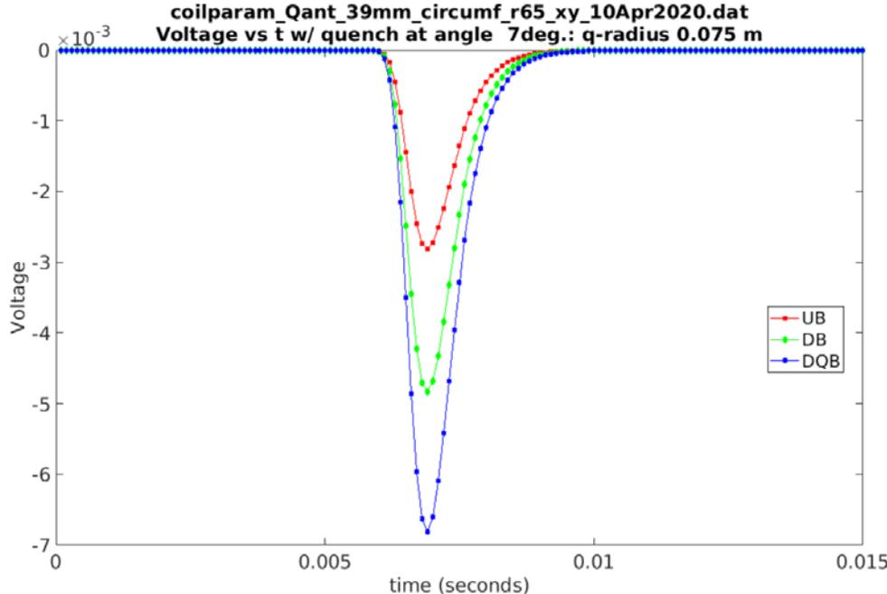
“parallel” Qant case: Quench is effectively at ~ +7 deg
