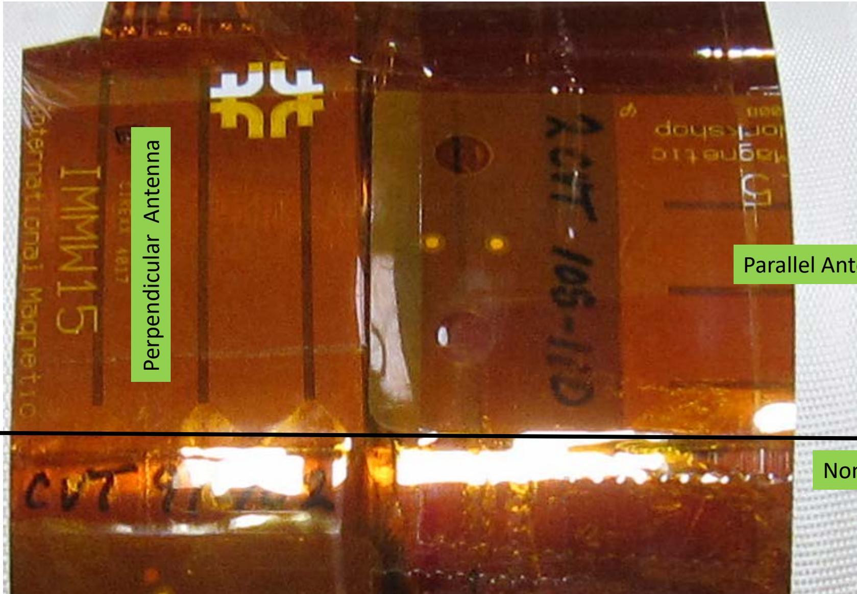
In the MQXFS1d Qant data, the perpendicular antenna data signals are in the noise, while the parallel antenna is always seen and has signal size of about 5mV. See if simulation matches these results:
