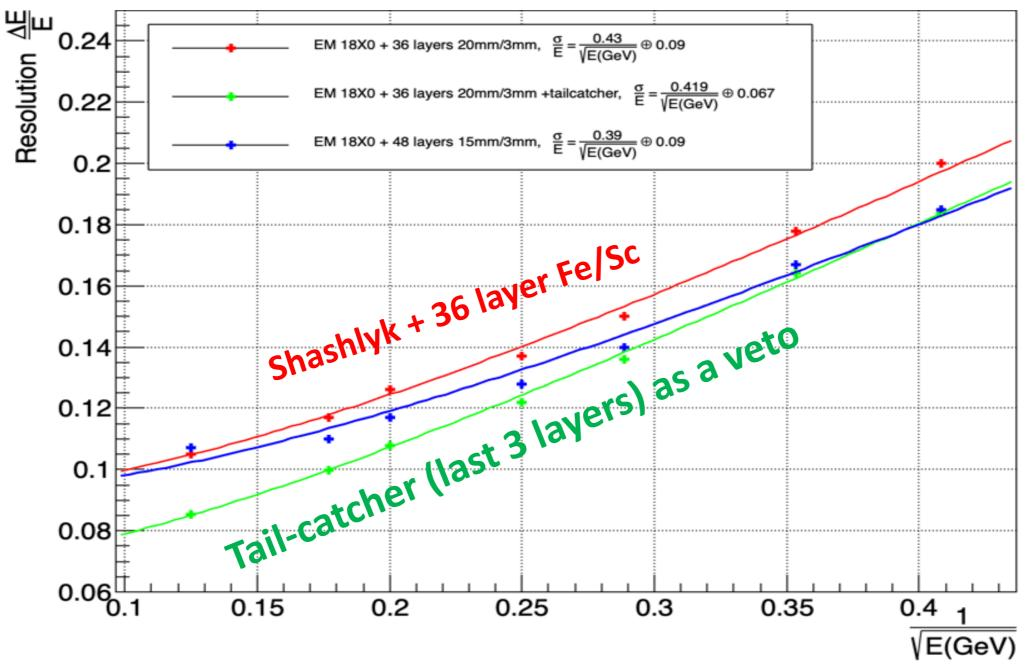
Tail-Veto – Improves energy resolution over all energy range **Detection Efficiency Loss:** 10% loss at 6 GeV; 50% loss at 64 GeV for charged pions
