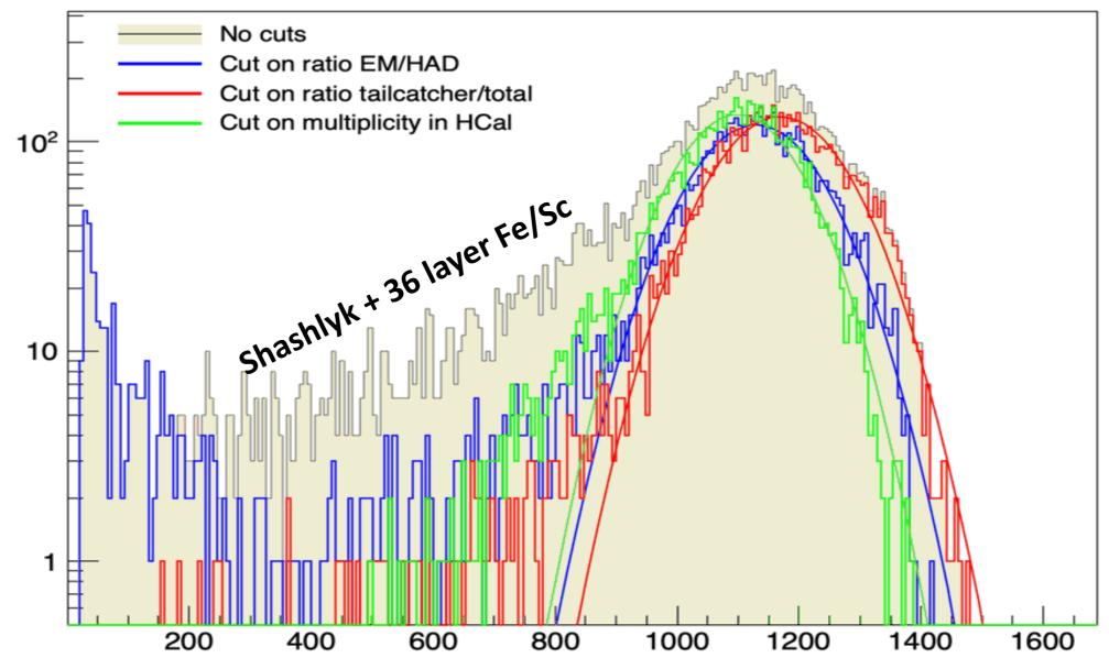
Tail-Catcher Method: Additional readout for last a few Sc plates Cut on HCal multiplicity Cut on EMCal/HCal energy ratio
