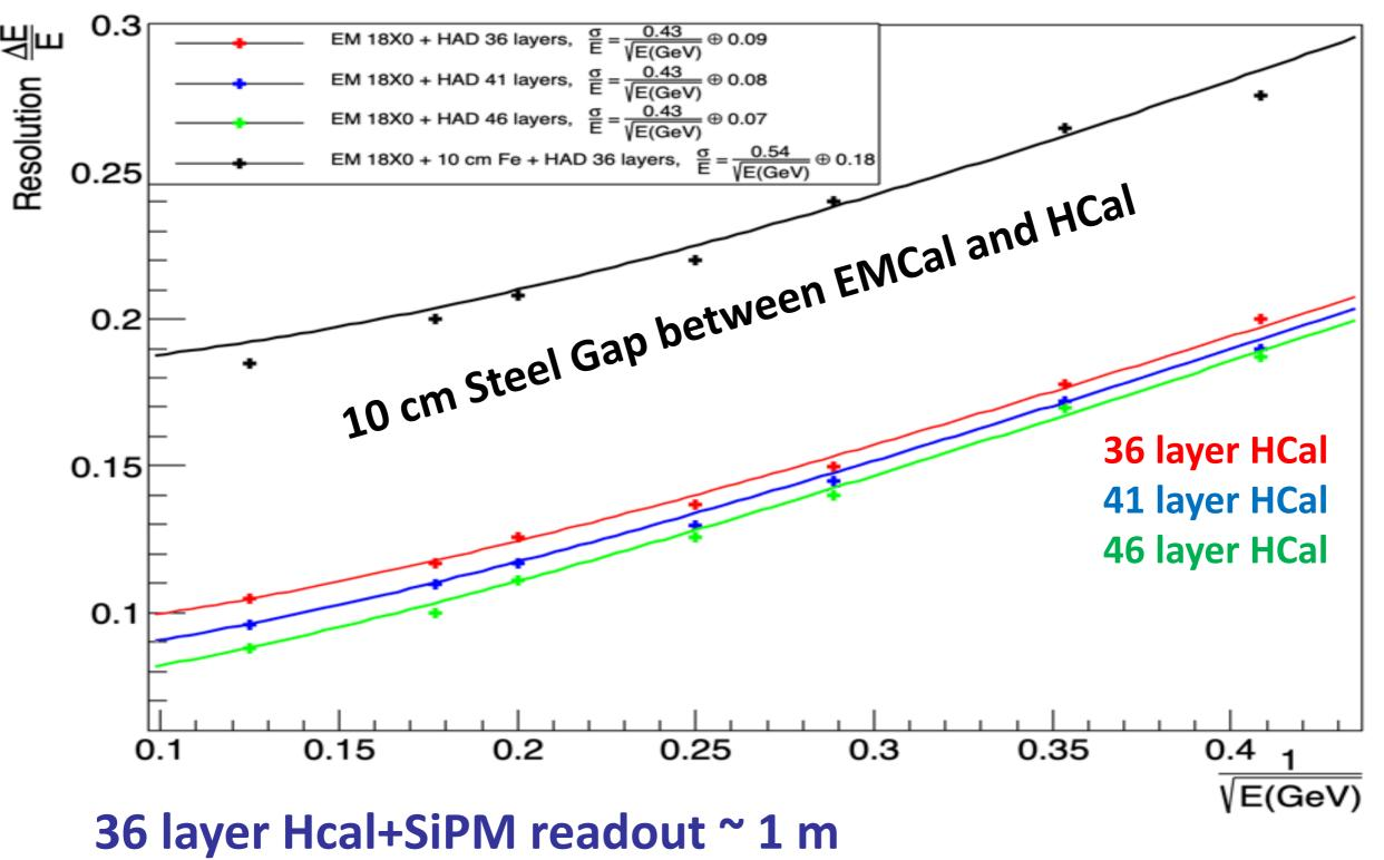
Mechanical Support for EMCal HCal -- important factor Energy leakage – unavoidable and more investigations
