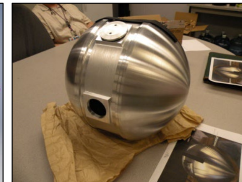
Target chamber for installation in the Gammasphere detector array
