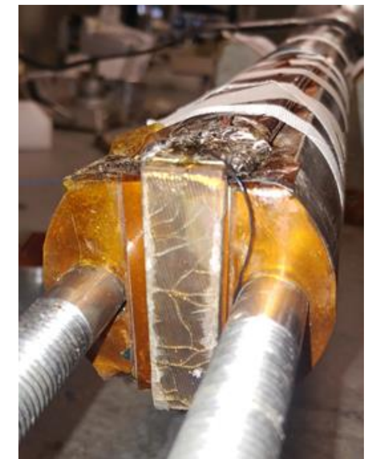
Sample after testing, as mounted to the fixture with the bottom pressure plate removed
