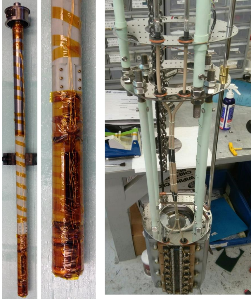
Sample holder, Pickup Coils, Dipole Magnet
