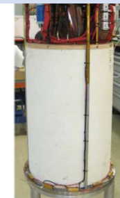
Fig. 2. Photo of the Oxford Instruments 20 T/78 mm bore LTS magnet outside its cryostat.
