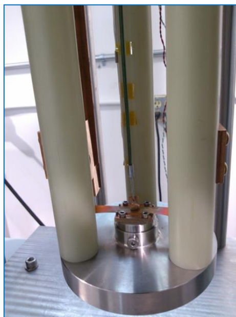
Transverse tensile Stud method RT or 77K w/ I_c
