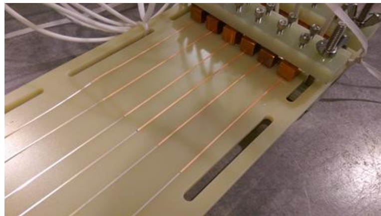
Selective Cu plated 1mm tapes under I_c test
