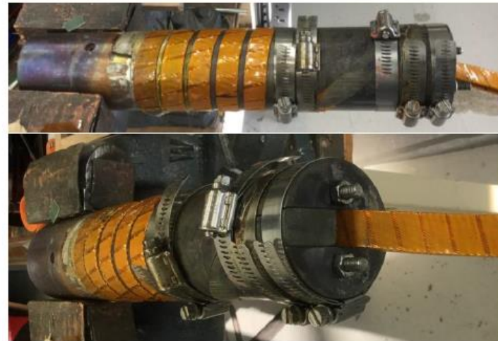
Fig. 10. NbTi cable sample assembly for MQE test of standard Rutherford cable and cable outfitted with high- C_p tape.
