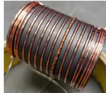
Fig. 3. Example of superconducting wire sample wrapped with Hyper Tech high- C_p tape cut down to \sim 1 mm width, along half a turn of the specimen.
