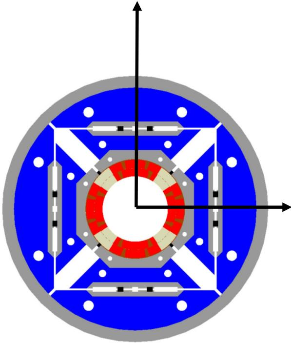
Quench Antenna T0 placed along Y-axis, s.t. Coil 113 lies between antenna signals T0 and T90
