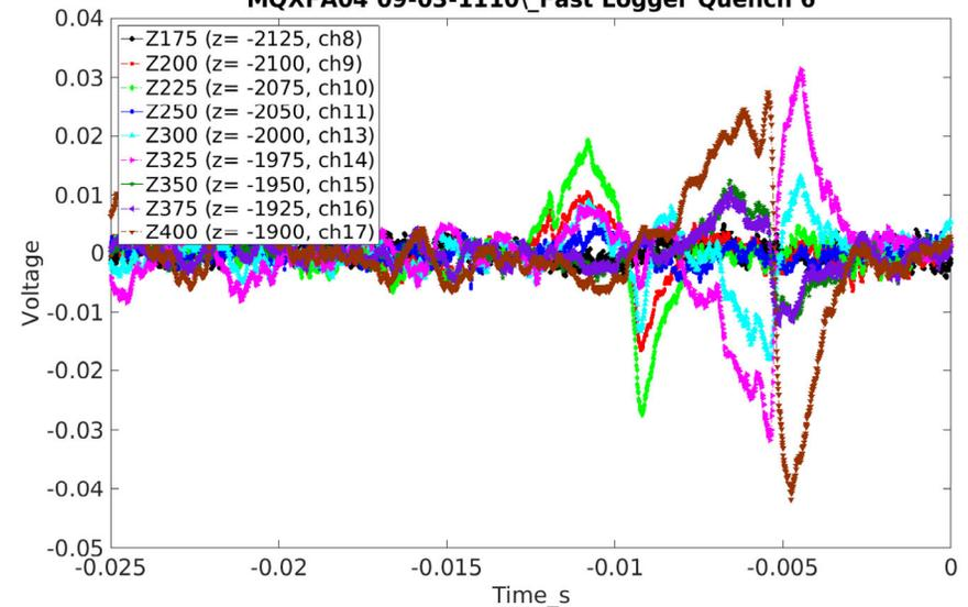
The QAA determined the Z-location of all recorded quenches to  $< 50\text{mm}$ .
