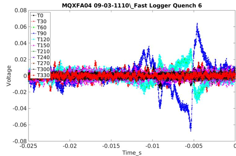
TQA quench activity was seen for all quenches and in the correct quadrant (and with relative intensity similar to that observed in ZQA).
