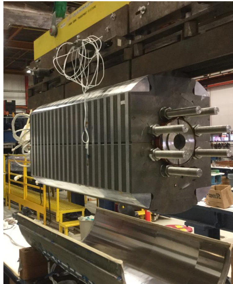
Transporting the iron yoke assembly from the shell to the clamping tooling
