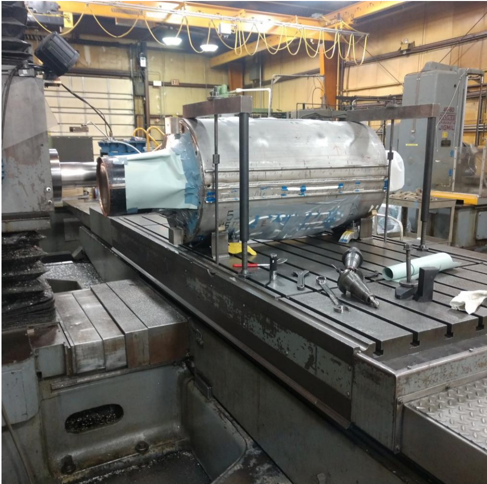
Magnet set up for the end ring cutting
