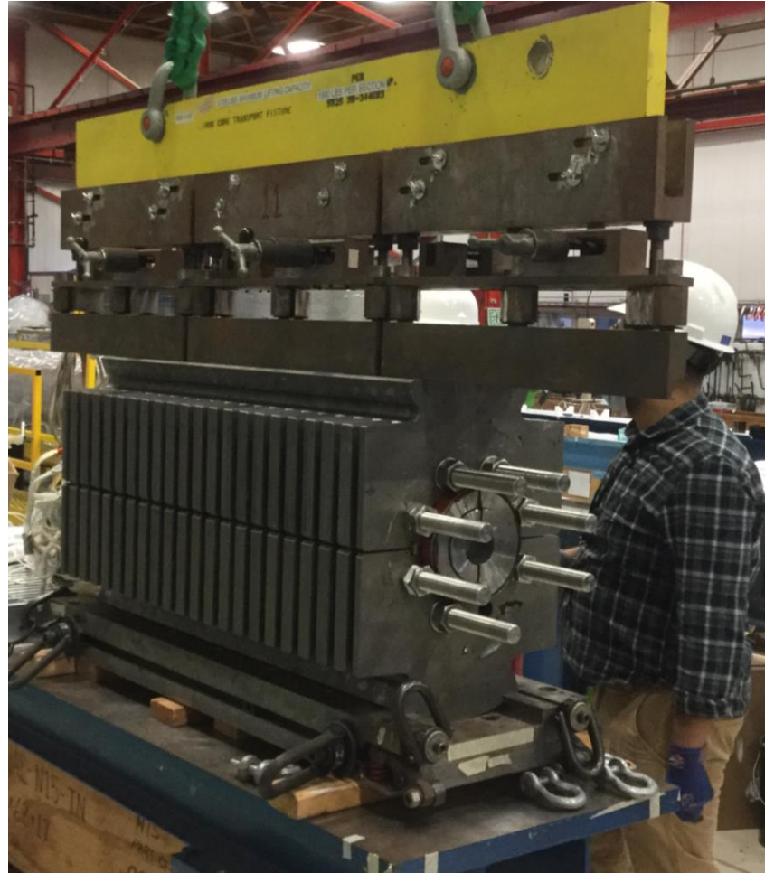
Lifting of the top iron yoke
