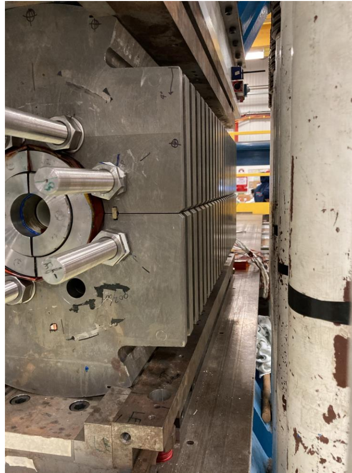
Magnet iron w/o clamps under press load
