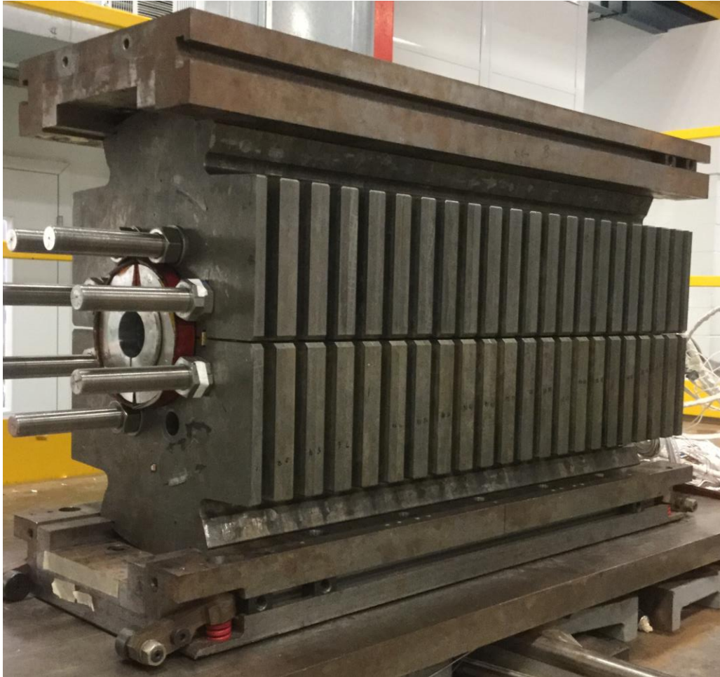
Iron yoke w/o clamps in clamping tooling
