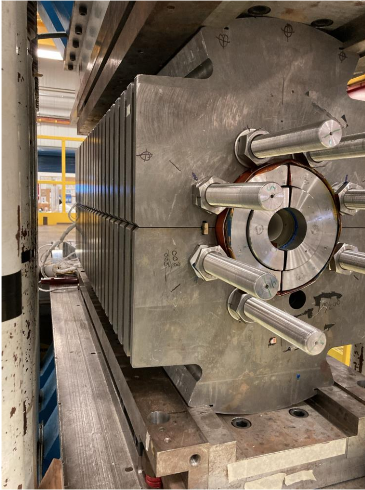
Magnet iron w/o clamps under press load
