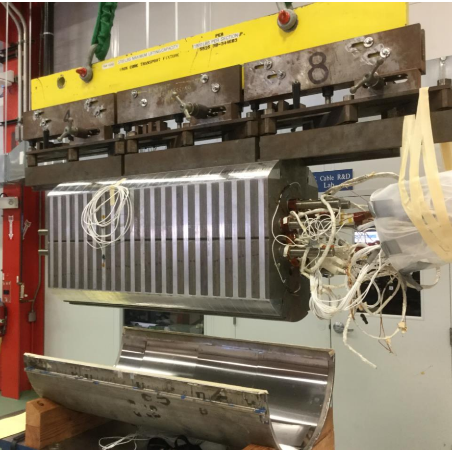
Transporting the iron yoke assembly from the shell to the clamping tooling
