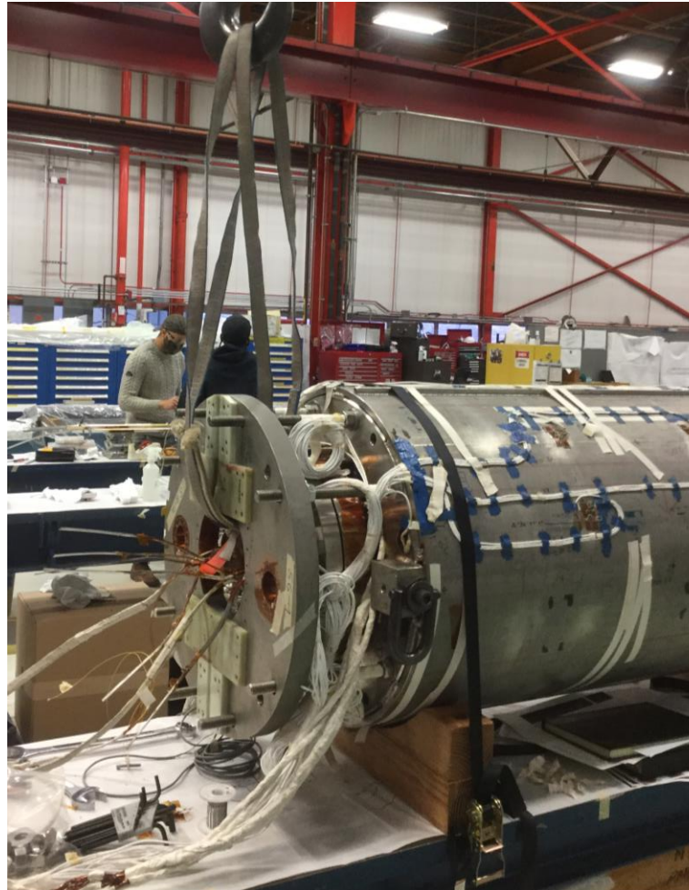
Lead's plate removal
