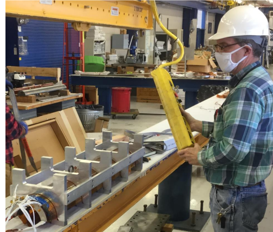
Outer coil in the holding fixture
