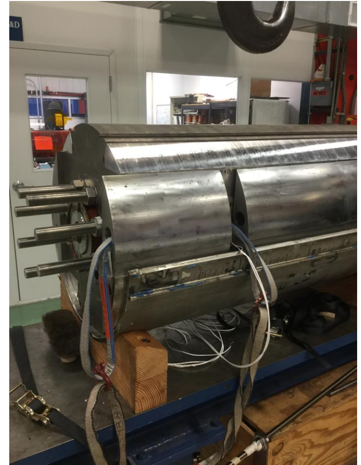
Removal of the yoke fillers
