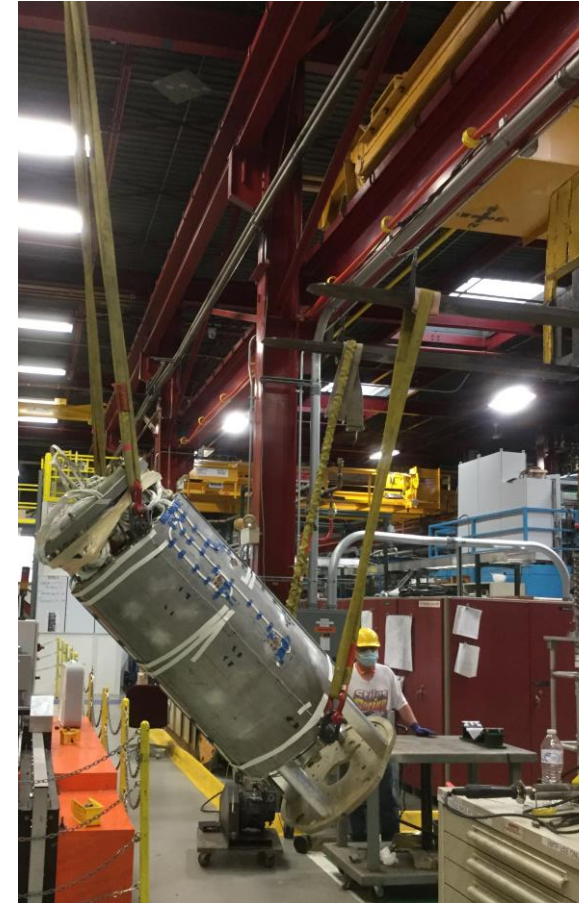
Magnet rotation procedure
