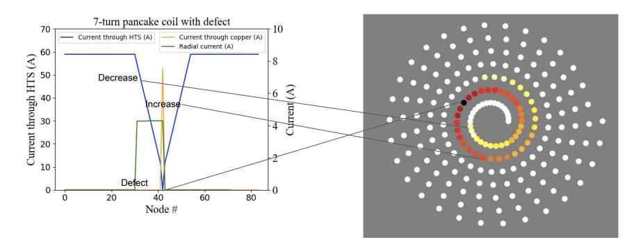
Current in HTS starts to decrease linearly from transport current level one turn before the defect, and increase linearly afterwards. It reaches the transport current level one turn after the defect spot.
