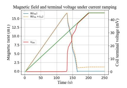
Simulation with operating current up to 100 A
