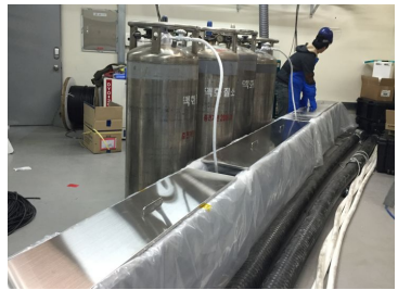
A 7 m single-phase 22.9 kV/50 MVA HTS cable (BSCCO)
