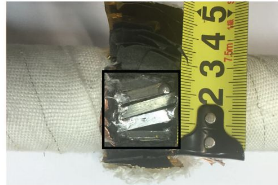
HTS cable's local insulation fault.
