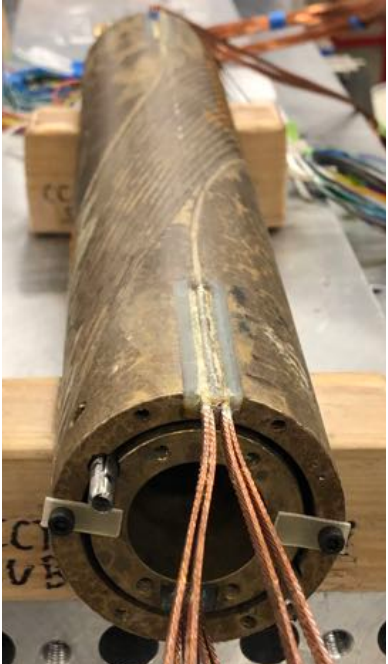
Layer 1/2 being assembled (w 45-degree Kapton bag)
