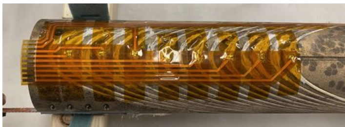
Voltage taps (32-ch SCXI/PCI w 18 bit ADC, 300Vrms isolation, programable gain and filtering)
