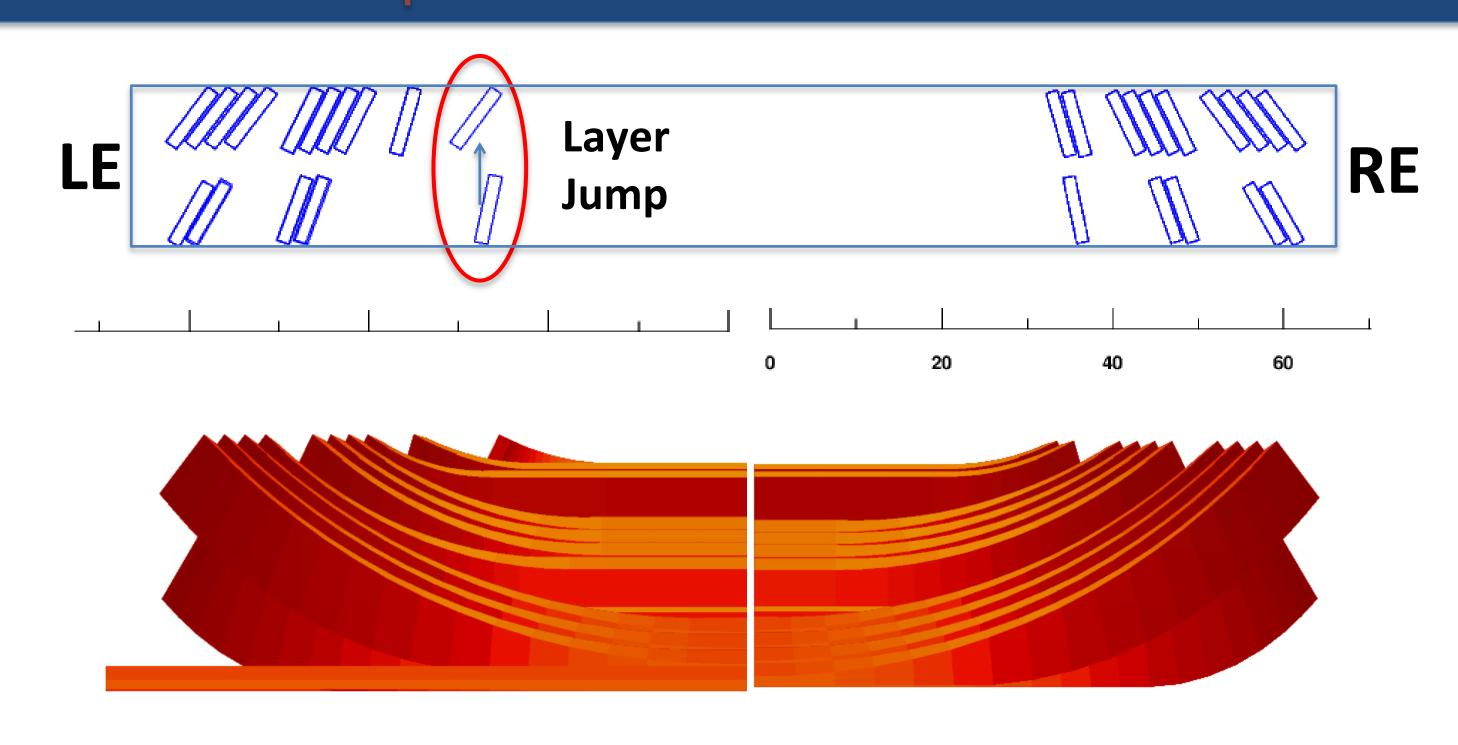
Layer jump approach: bend inner cable up to match the outer layer cable angle
