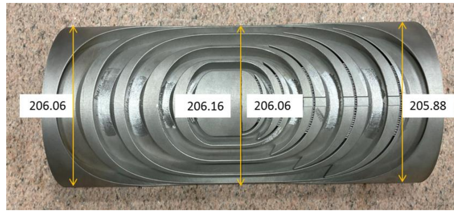
Control of SMCT coil end parts by micrometer on granite table.
