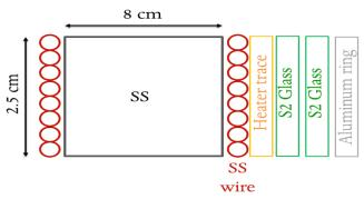
Use small solenoid made of cheap NiCr or NbTi leftover wires:
