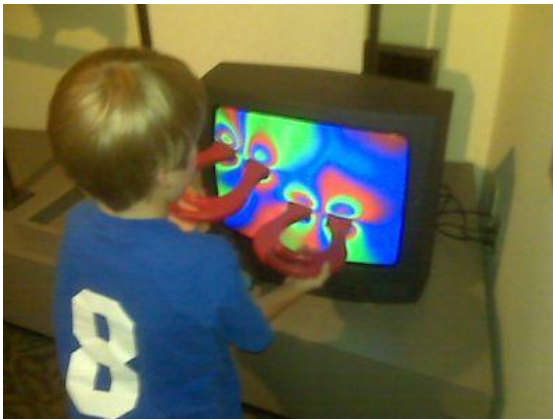
Distorted TV picture from electrons taking a curved path in the presence of a magnetic field
