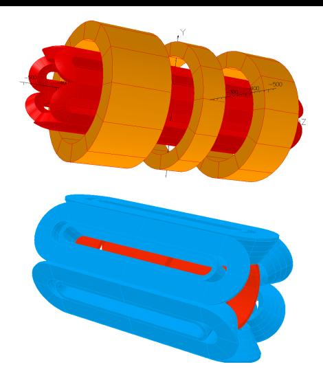
VENUS and SECRAL-II have reached limits of NbTi superconductor in these two coil configurations
