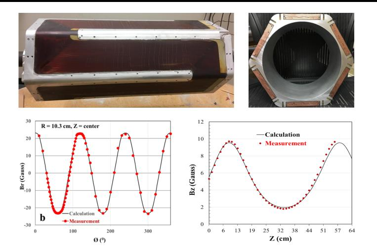
The closed-loop-coil is difficult to wind. To address this:
