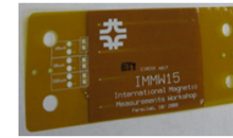
Figure 5.3 – Quench antenna on a "trace" with three channels (left) and simplified drawing (right) of the proposed 2D-grid with quench antenna sensors. The grid could be 3D with the addition of a differently designed antenna placed in depth along the cable (a much more complicated option).
