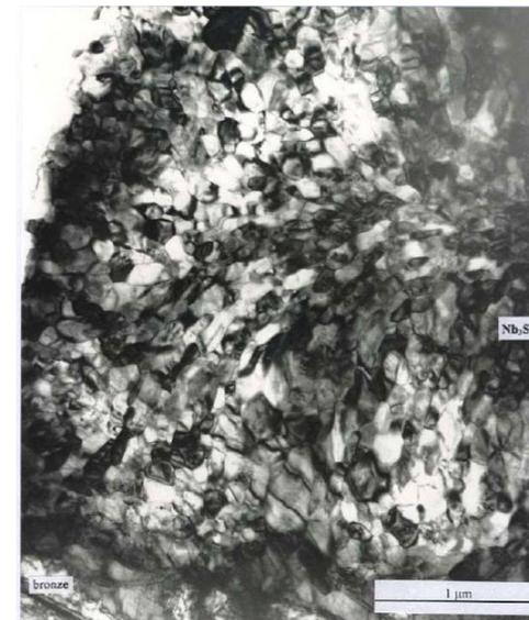
Fig. 6: Microstructure of a Nb<sub>3</sub>Sn filament (Courtesy of C. Verwaerde, Alstom/MSA).
