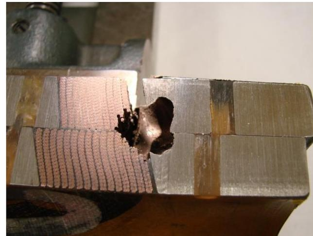
Quench-related damage in the coil of HQ01 quadrupole
