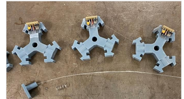
Various AE sensors and mounting hardware (LBNL)
