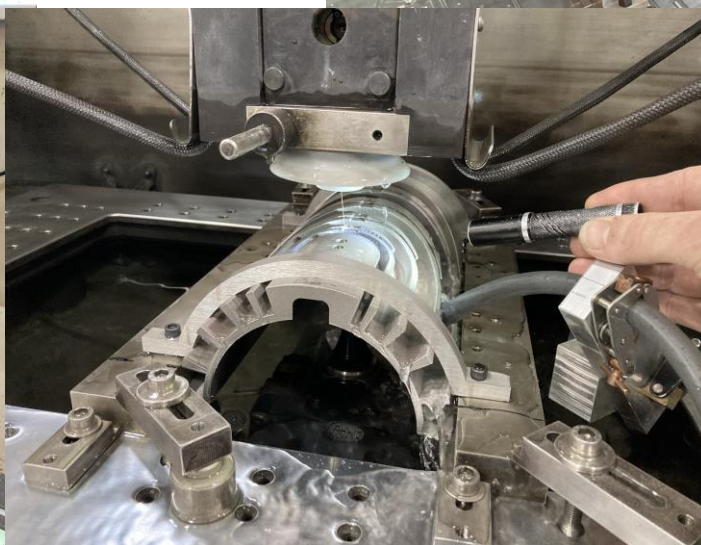
Wire EDM set up with new rotation head
