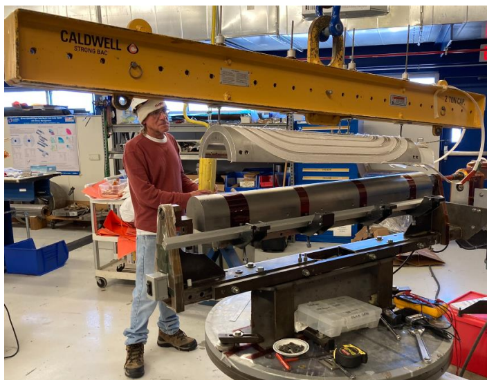
Lifting coil up from the winding table
