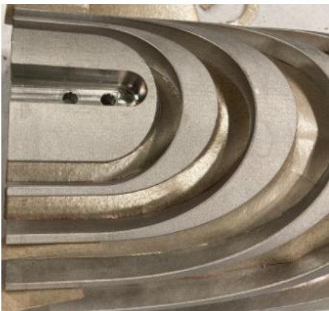
Mica and S2 glass strips for the groove insulation
