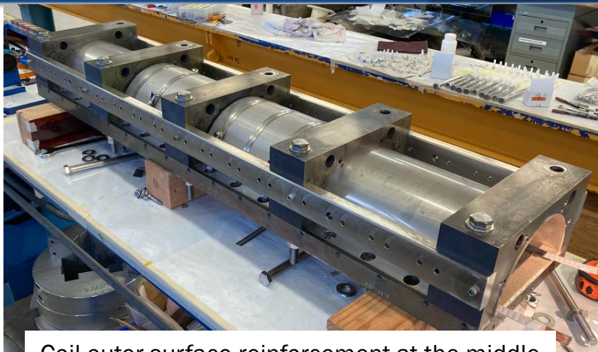
Coil outer surface reinforcement at the middle
