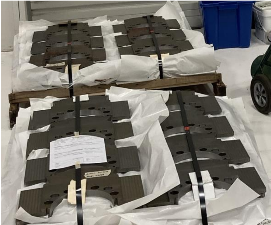
Iron laminations after modification
