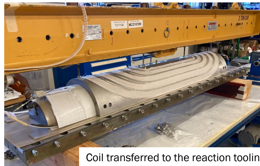
Reaction mandrel and bottom plate with Mica insulations
