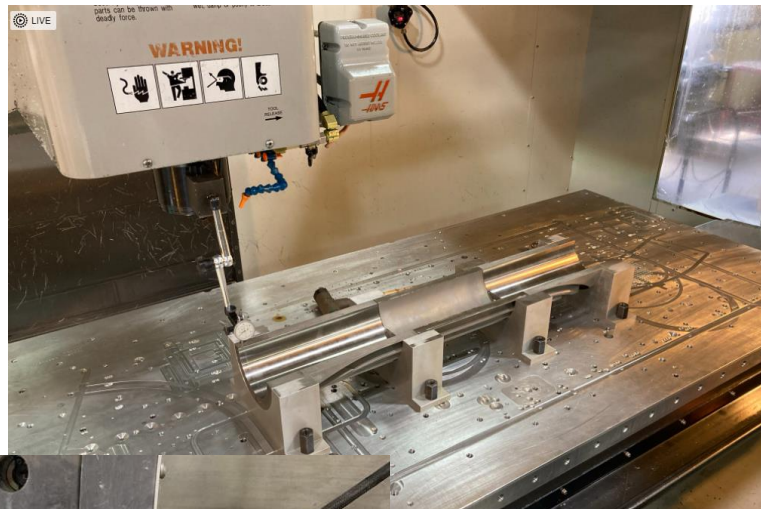
Central part machining setup and dimensional control
