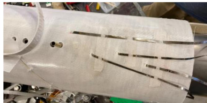
L1 VT strips located between two inter-layer blankets
