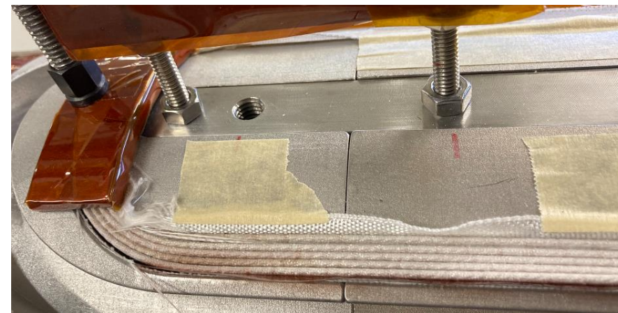
First groove insulation scheme for L1 and real winding of L2
