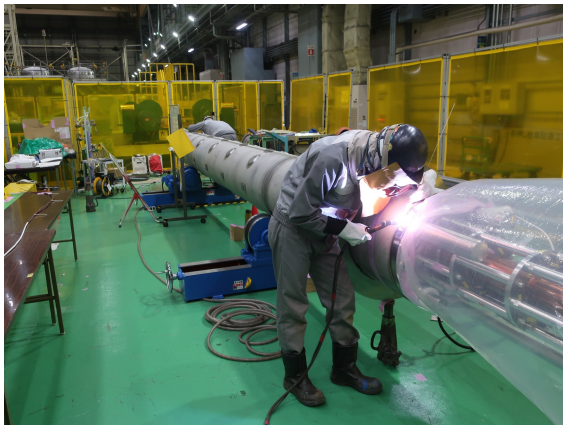
End Dome Welding
