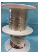
Wires identified and shipped from LBNL to KEK for testing KEK's new ceramic coating insulation on \text{Nb}_3\text{Sn} and Bi-2212 wires.
